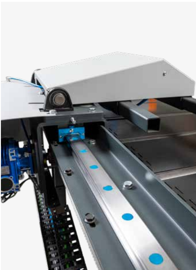
Motorized measuring device assembled on a 45mm linear guide and 4.7Nm servo motor.
