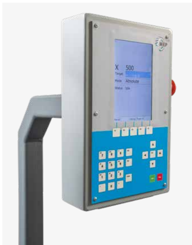
Turning control panel with 7" display mounted on a free-standing base and equipped with piece counter, blade kerf compensation and device for remote programming via ethernet cable.
