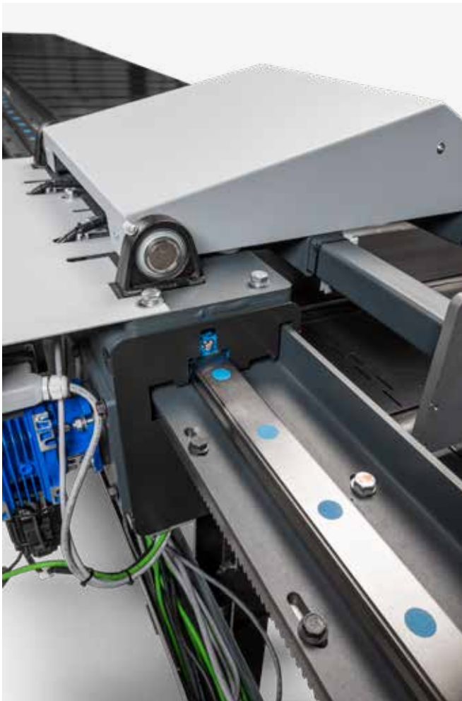
Motorized measuring stop device assembled on 45mm linear guide and 4.7Nm servo motor.
